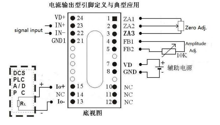
Current Signal Output Transmitter PIN Description: DIP 24 Pin Package with Gain/Zero Adjustment
