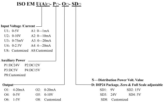
Note: If SD does not required, that is distribution power is not required in use, user can omit that functions 5VDC distribution or does not connect the pins for distribution power when using it.
