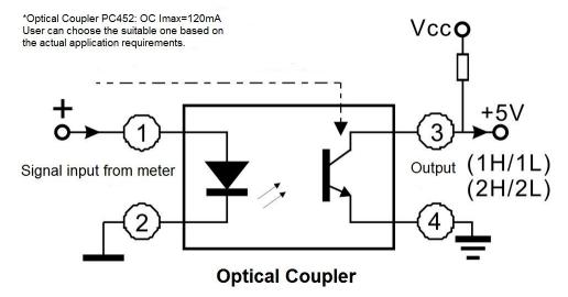
3. Due to the max. current limit of photosensitive triode IC, the capability of the meter in current amplification and drive load is limited. If the greater drive current is required to propel inverters, magnetic valves, stepper motor or other devices, user can add power expansion circuit (power amplifier tube or servo circuit) to amplify current or order it from us specially.
