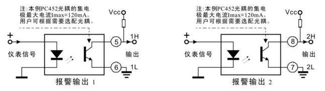
3. Due to the limitation of the maximum current of the phototransistor Ic, its current expansion and drive load capacity are limited. If users need more drive current to drive relays, solenoid valves, stepping motors and other devices on site, they can connect external power expansion circuits by themselves (Power amplifier tube or servo circuit) for expansion and amplification processing or special customization.
