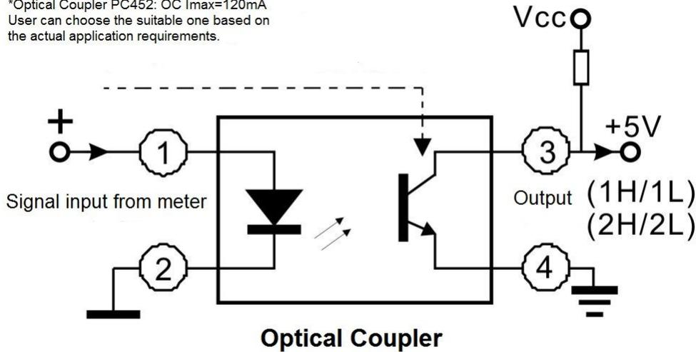
3. Due to the max. current limit of photosensitive triode IC, the capability of the meter in current amplification and drive load is limited. If the greater drive current is required to propel inverters, magnetic valves, stepper motor or other devices, user can add power expansion circuit (power amplifier tube or servo circuit) to amplify current or order it from us specially.
