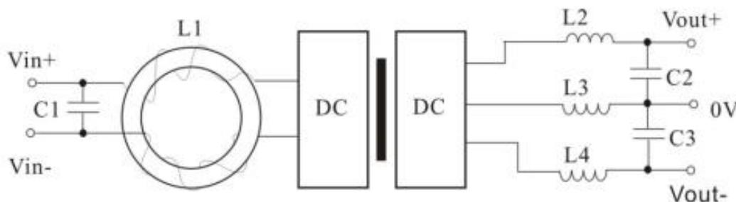
三. DC-DC module converter isolation withstand voltage test method
