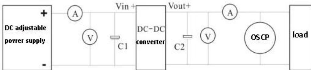
二. Reference method for reducing noise common mode interference in the use of DC-DC module converter.
