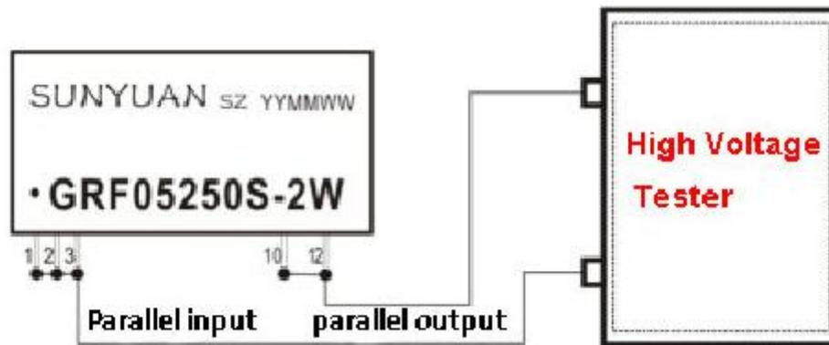
**Safety precautions and conventional methods of product high voltage isolation test:**
