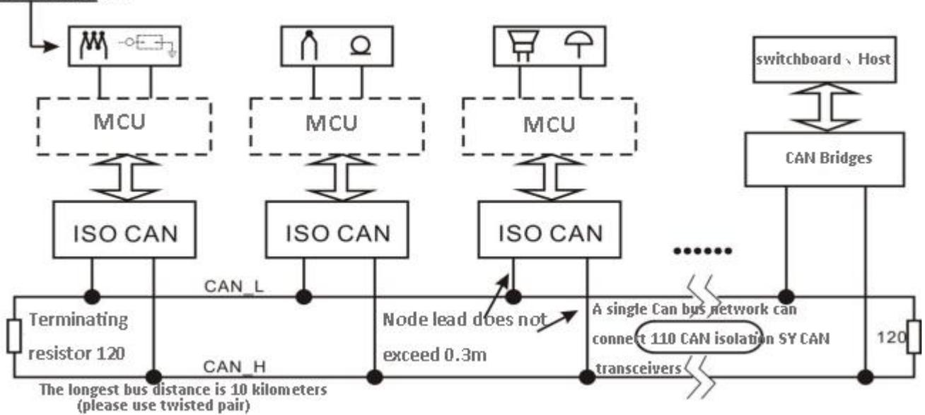
A typical CAN-bus network is shown in the figure above. Each network can be connected to 110 single-channel ISO CAN isolation bus transceiver modules. The longest communication distance of the universal module is 10km, and the high speed module supports the lowest baud rate of 40kbps and the longest communication distance. 1km. If you need to access more nodes or a longer communication distance, it can be expanded through CAN interrupters and other devices.
